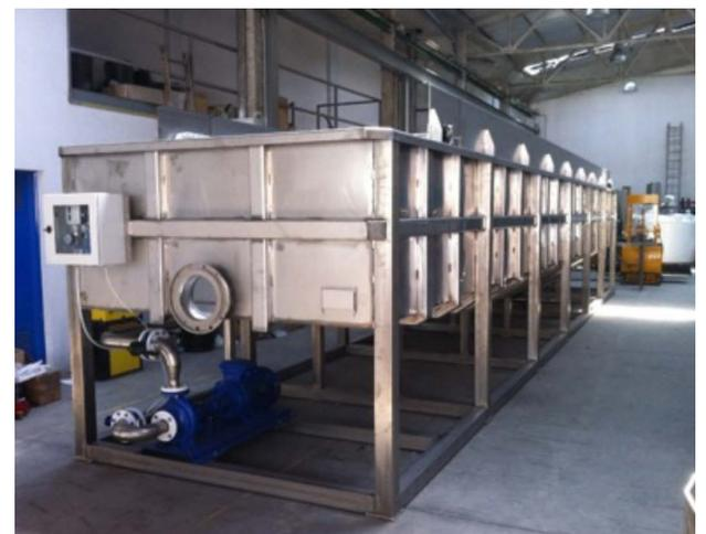
SIGMADAF was contracted by PROMARINA for the design-supply of the equipment to be installed at the existing ETP including pre-flotation for separation of oil
